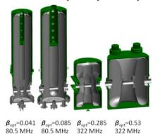
Figure 3: SC Quarter-Wave Resonators and Half-Wave Resonators used in FRIB SC linac Segments 1 and 2.
