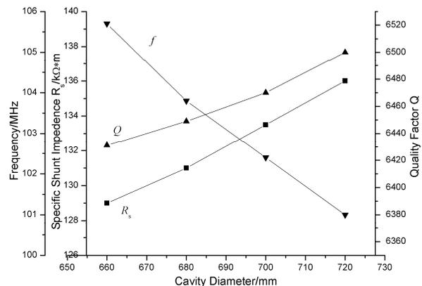
Figure 6: Sensitivities of resonant frequency, transverse shunt impedance and quality factor of the T-IH-RFQ to cavity diameter.
