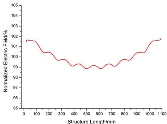
Figure 7: Longitudinal flatness of electric field.
