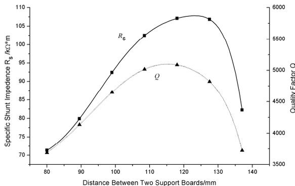
Figure 4: Transverse shunt impedance and quality factor of the T-IH-RFQ as a function of the distance between two neighbouring support boards.
