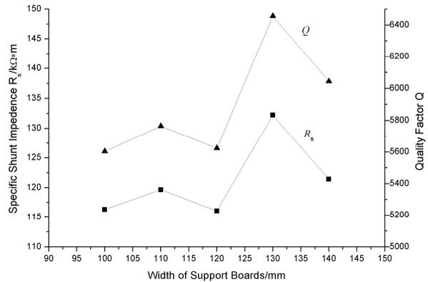
Figure 5: Transverse shunt impedance and quality factor of the T-IH-RFQ as a function of support board width.
