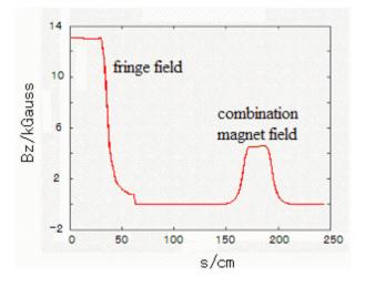
Figure 1: Magnetic field along the extracted beam path.
