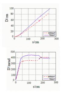
Figure 3: Beam dispersions at 70 MeV and 100 MeV.
