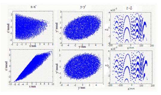
Figure 4: Distribution of 100 MeV particles at the stripper and the exit of the combination magnet .
