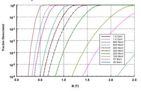
Figure 1: Fractional Lorentz stripping over a 1 m path for various energies as a function of B.
