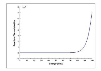
Figure 2: Dissociation of H<sup>-</sup> as a function of energy in the CYCIAE-100.
