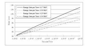
Figure 3: H<sup>-</sup> beam loss versus N<sub>2</sub> equivalent pressure.
