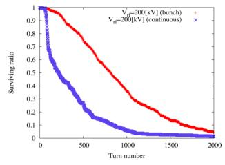
Figure 4: presents the particle survival as a function of turn number.
