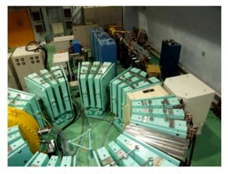
Figure 5: Photograph of FFAG-ERIT accelerators.
