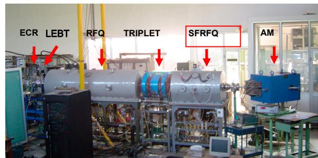
Figure 1: Accelerator system composed by ISR-RFQ 1000 and SFRFQ.
