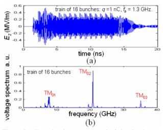
Figure 3:  $E_z$  at the downstream end of the decelerator, excited by a train of 16 bunches. (a) E-field; (b) voltage spectrum.
