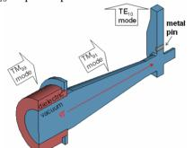
Figure 5: CST Microwave Studio model of the 35.1GHz  $TM_{03}$ -TE<sub>10</sub> output coupler.
