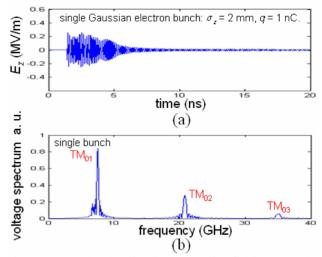
Figure 2: The longitudinal electric field  $E_z$  at the downstream end of the decelerator, excited by a single bunch. (a) E-field; (b) voltage spectrum.
