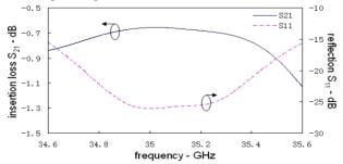
Figure 7: Simulated S-parameters of the 35.1GHz  $TM_{03}$ - $TE_{10}$  output coupler.
