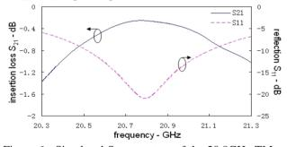
Figure 6: Simulated S-parameters of the 20.8GHz  $TM_{02}$ -TE<sub>10</sub> output coupler.
