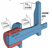
Figure 4: CST Microwave Studio model of the 20.8GHz  $TM_{02}$ -TE<sub>10</sub> output coupler.
