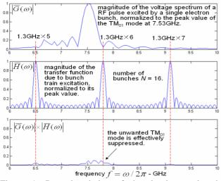
Figure 1: Properly choice of the decelerator length effectively suppresses the unintended  $TM_{01}$  mode. The train consists of 16 electron bunches in this case.
