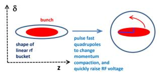
Figure 1: Schematic of fast bunch rotation in a storage ring.
