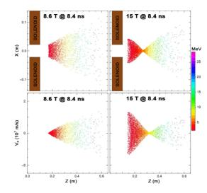
Figure 9: Warp simulations: (top) transverse deflection X and (bottom) transverse proton velocity  $V_x$  versus beam propagation direction Z for two different magnetic field strengths 8.6 T and 15 T at the time 8.23 ns. Injected proton energies: (2.3-28.7) MeV.
