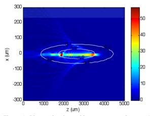
Figure 1: Plasma density and beam contour plot at z=1cm. The plasma electron density color map is normalized to the uniform plasma density  $n_p$ . The two contours show the 10% and 90% beam charge levels.
