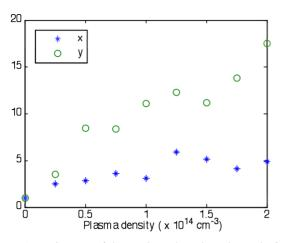
Figure 4: Emittance of the positron bunch at the end of the 1.4 m long plasma as a function of the plasma density.
