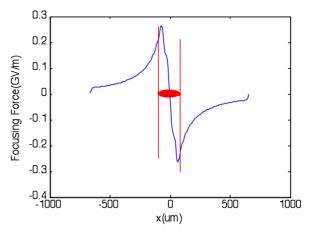
Figure 2: plasma focusing force on the e beam at z=1 cm for  $n_p=10^{14}$  cm<sup>-3</sup>, evaluated in the middle of the bunch ( $z=2500 \mu m$  on Fig.1).
