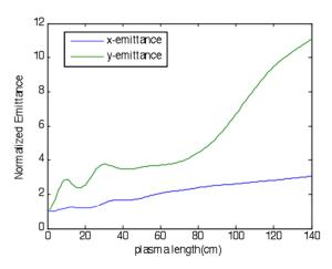
Figure 3: emittance growth of positron bunch along the plasma. The normalized emittances (see Eq. 1) are also normalized to their values at the plasma entrance.
