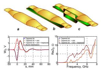
Figure 3: Simplified model of IR-extraction chamber. a) Tapered elliptic chamber. b) Tapered elliptic chamber with narrow slot. c) Tapered elliptic chamber with narrow slot and trapezoidal slot. **Left Bottom:** The longitudinal shortrange wakepotential for a 3mm Gaussian bunch. **Right Bottom:** The real part of the longitudinal impedance.
