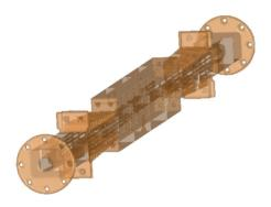
Figure 2: VORPAL screenshot showing the collimator structure.
