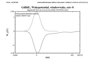
Figure 5: Transverse wakefields excited by a bunch of 1 mm in a complete collimator with closed jaws.
