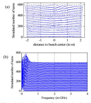
Figure 3: Mountain range of the time domain (a) and frequency domain (b) simulated delta signals of a long debunching bunch interacting with a the resistive wall model of the SPS kickers impedance.
