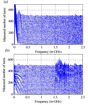
Figure 4: turn-by-turn mountain range of the measured sum (a) and delta (b) frequency spectra of a long unstable debunching bunch in the SPS measured with BPW 31901.
