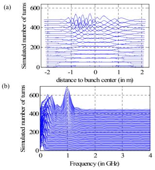
Figure 2: Mountain range frequency spectrum of the simulated vertical delta signals of long debunching bunch interacting with dipolar and quadrupolar contributions of a broadband impedance (flat pipe).
