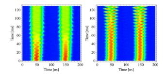
Figure 1: Last two bunches of the 18 bunch batch on the flat-top. The second harmonic (h=42) is increased to 16 kV within the first 70 ms (left). The SH case (h=21 only) is shown on the right plot.
