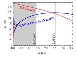
Figure 3: Synchrotron frequency versus single particle emittance for single and DH RF system (voltage ratio 0.5). A bunch of  $\varepsilon_l = 1.4\,\mathrm{eVs}$  covers the gray shaded area. A phase error of  $0^0$ ,  $2^0$ ,  $4^0$ ,  $6^0$ ,  $8^0$ ,  $10^0$  (from bottom to top trace) has been assumed between the two RF systems.
