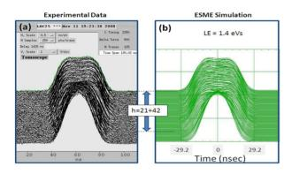
Figure 2: Comparison between (a) measured and (b) simulated mountain range pictures during flat bunch formation.
