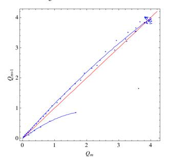
Figure 3: "bunch-by-bunch" electron dose map  $Q_{m+1}$  vs  $Q_m$ . Circle markers: ECLOUD simulations ( $\delta_{max}=1.8$ , all other parameters as in Table I). The red line represents saturation ( $\rho_{m+1}=\rho_m$ ). Markers above the saturation line describe the buildup. Markers below the saturation line describe the e-cloud decay. The blue lines are the corresponding cubic fits. Transitions between filled and empty bunch trains are shown as black circles.
