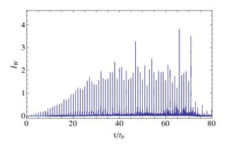
Figure 1: Instantaneous current  $I_W$  of electrons bombarding the wall of an LHC arc dipole computed with ECLOUD. The case shown corresponds to a filling pattern featuring 72 charged bunches, with bunch charge of  $N=1.8\cdot 10^{11}$  protons, followed by 8 empty (zero-charge) bunches. The assumed bunch spacing is 7.48 m, and the SEY is  $\delta_{max}=1.8$ .
