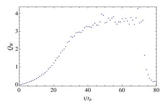
Figure 2: "bunch-by-bunch" electron dose  $Q_m$ . The case shown corresponds to a filling pattern featuring 72 charged bunches, with bunch charge of  $N=1.8\cdot 10^{11}$  protons, followed by 8 empty (zero-charge) bunches. The assumed bunch spacing is 7.48 m, and the SEY is  $\delta_{max}=1.8$ .
