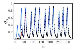
Figure 4: Electron dose "bunch-by-bunch" evolution for two different bunch-train filling patterns, for  $N=1.8\cdot 10^{11}$  and  $\delta_{max}=1.8$ . Top: (24f,12e,36f); bottom:  $3\times (12f12e)$ . In both cases, successive bunch trains are separated by gaps whose length corresponds to 28 (empty) bunches. Black markers: ECLOUD results. Blue and red lines: map results corresponding to different initial electron doses.
