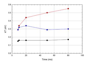
Figure 4: For a plasma that experiences no evaporative cooling,  $kT_{\perp} = 0.17 \text{ eV}$  (black), but  $kT_{\perp} = 0.30 \text{ eV}$  for a plasma where evaporative cooling occurs between t = 7 ms and 10 ms (blue). If the cooling is applied permanently at t = 7 ms, then  $kT_{\perp}$  continues to grow with time (red).
