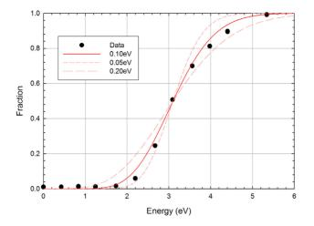
Figure 3: The measured on-axis charge that remains trapped (black dots) drops to zero as the axial-trapping barrier is reduced to zero. The rate of change in the on-axis charge is consistent with an axial temperature of 0.1 eV when the axial distribution is assumed to be a drifting Maxwellian with a mean velocity corresponding to 3.1 eV (solid red line).
