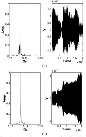
Figure 4: Simulated beam spectrum and dipole oscillation in vertical plane for different bunch current: (a) 0.69 *mA*; (b) 0.70 *mA*. Bunch length is 3mm.
