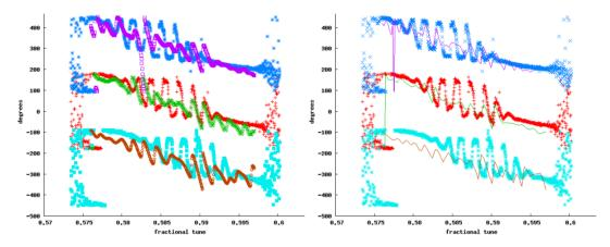
Figure 2: Horizontal phase BTF response of a chromaticity measurement +40Hz (top), -40Hz (bottom) and zero Hz middle. Simulation overlaid on actual data. Horizontal Chromaticity is set to 8.5 units. Left plot with wake fields, right plot without.
