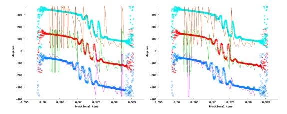
Figure 3: Vertical phase BTF response of a chromaticity measurement +40Hz (top), -40Hz (bottom) and zero Hz middle. Simulation overlaid on actual data. Vertical Chromaticity is set to 4 units. Left plot with Wakefield, right plot without.
