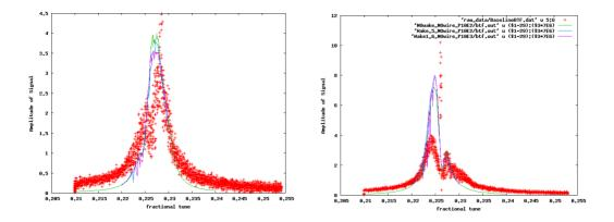
Figure 1: Impact of various Wakefield strengths on the vertical amplitude response of a BTF simulated measurements compared with actual.
