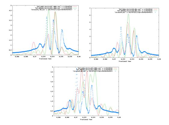
Figure 4: Vertical amplitude BTF response for a chromaticity measurement. Simulation overlaid on actual data. Vertical Chromaticity is set to 4 units. Blue trace is actual, green simulation without wake and red simulation with wake fields. Plots left to right (-40Hz,0, +40Hz)
