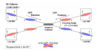
Figure 3: Crab cavity correction for Super-KEKB.
