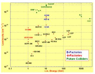
Figure 12: Peak luminosity of various colliders showing the proposed Super-KEKB and Super-B approaching 10<sup>36</sup>. (Courtesy of M. Biagini.) acknowledgments.
