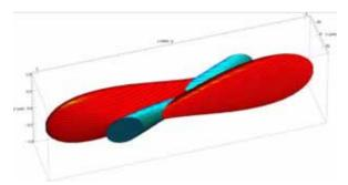
Figure 5: IP beam sizes with Crab Waist correction.
