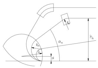
Figure 4: Scheme of the 180° bends with two magnets.
