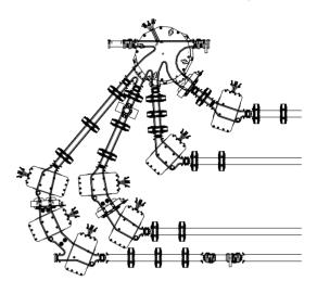
Figure 5: Magnets and vacuum chamber of bends.
