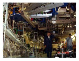
Figure 6: The bends are hanged on the ceiling. Round magnet is at the top left corner, the old teraherts FEL magnetic system is at down-left. Elements of the optical resonator for the second-turn FEL are yet at the floor (down-right corner).
