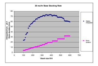
Figure 4. Integrated Luminosity as a function of the stash size at a  $30 \times 10^{10}$ /hr antiproton production rate (ZSSR).
