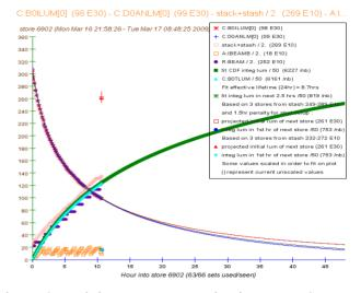
Figure 6. Real-time Tevatron Luminosity Decay Summary plot, used in daily operations to help determine the store termination time.
