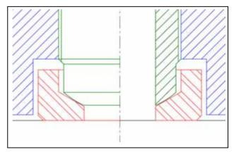
Figure 1: The leg consists of the fine-thread screw and the horseshoe-part.
