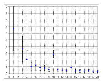
Figure 4: The statistical results of  $\sqrt{A_n^2 + B_n^2} / \sqrt{A_2^2 + B_2^2}$  for the first twenty harmonics on 114 serial quadrupoles at 150A. In units 0.0001.
