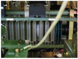
Figure 6: Switching thyristor of the power supply.
