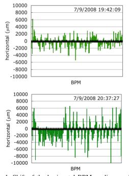
Figure 1. Shift of the horizontal BPM reading produced by an anomalous cycle performed on the main dipoles of sector 2-3. The beam travels from left to right through three sectors, from point 2 (left-most) up to point 5 (rightmost). The anomalous pre-cycle in sector 2-3 inverts the magnetization, increases the integral dipole field, and shifts the orbit inwards by an average of 1.4 mm (first third of the series of BPM readings).
