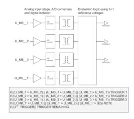
Figure 1: Symmetric quench detection functional circuit diagram.
