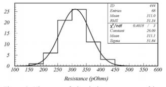
Figure 4: Histogram of electrical measurements of bus splice resistances.
