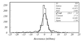
Figure 6: Histogram of electrical measurements of internal magnet splice resistance differences.
