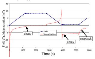
Figure 1: Calculated magnetization change of the strands in a 2.2m long 14 strand Rutherford cable.
