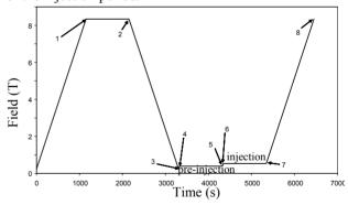
Figure 3: Typical LHC pre-cycle.
