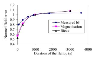
Figure 6: Comparison of calculated BICCs and magnetization decay with the measured sextupole decay.
