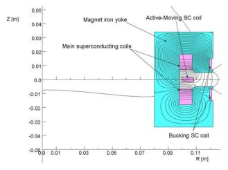
Figure 3: Magnet cross-section and flux lines.
