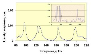
Figure 6: Cavity-tuner system transfer function. Active coil exited with sine wave current drive signal. Frequency of drive signal swept from 20 Hz up to 700 Hz.
