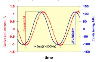
Figure 7: Tuner fast mode of operation. The active coil current is (f = 200 Hz and Ia = 2A), Im = 30 A.
