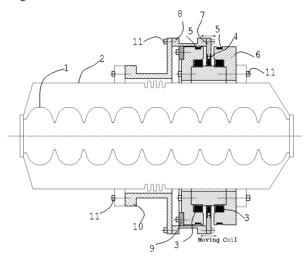
Figure 1: Electromagnetic Tuner cross-section.
