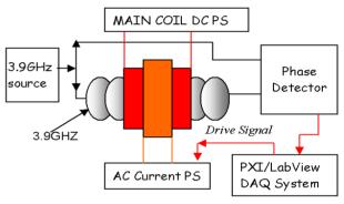
Figure 4: Phase detection scheme.
