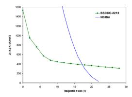
Figure 1: J<sub>E</sub> vs. B for Nb<sub>3</sub>Sn and Bi-2212 wires.
