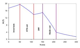
Figure 5: Maximum field in HS coil cross-section as function of the radial direction. No correction coil.
