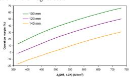
Figure 4: Operational margin as a function of superconductor (Bi-2212) engineering current density.
