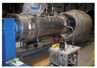
Figure 3: Cold mass ready for installation.
