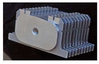
Figure 5: A 10-pole prototype manufactured using an Al core and the assembled technique.
