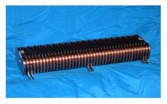
Figure 6: A 42-pole test coil wound on an assembled iron-core with iron poles.
