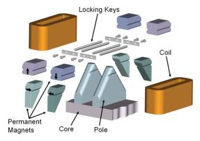
Figure 2: Exploded view assembly.
