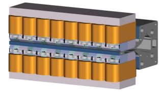
Figure 1: Circular polarizing quasi-periodic undulator (only four periods shown).
