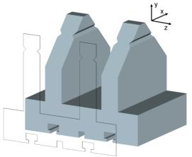
Figure 4: Configuration for a laminated core.
