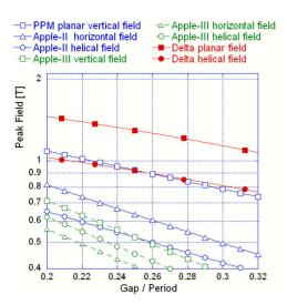
Figure 2: Peak field as a function of gap to period ratio for various types of undulators.
