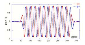
Figure 5: Horizontal and vertical field components measured along beam axis in helical mode. wave fit applied to the horizontal and vertical field components gave 0.873T and 0.856T for the field amplitudes and  $88^0$  phase between them. The measured field amplitude is  $\sim 13\%$  less than was predicted by calculation. The cause of the field amplitude reduction was found to be the imperfection in the mechanical structure. In the next version of the model it will be fixed.
