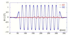
Figure 7: Two orthogonal field components measured along the magnet in planar mode.
