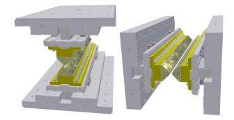
Figure 1: Two pairs of magnet arrays forming Delta undulator structure. On the left side are arrays generating vertical field, on the right - horizontal.
