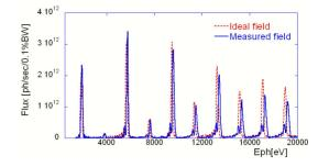
Figure 8: X-ray flux spectrum for the measured and ideal fields in planar mode.
