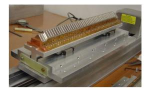
Figure 4: Magnet array on the field measurement bench.
