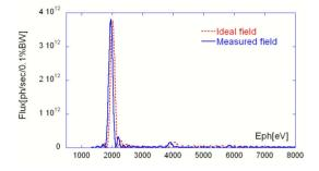
Figure 6: X-ray flux spectrum calculated for the measured and ideal fields in helical mode.
