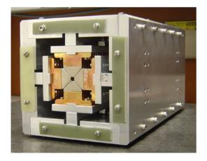
Figure 3: Partially assembled model with visible magnet arrays.
