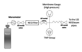
Figure 3: Schematic of the Ne injection line.
