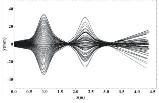
Figure 4: The trajectory of 100 particles in the vertical plane between the cyclotron and the FFAG ring, as obtained by GPT package. Two waists in the middle and at the end of the longitudinal direction correspond to the place where a buncher may locate and the entrance of the FFAG ring.
