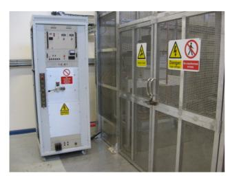
Figure 4: The platform bias DC power supply and the high voltage cage.
