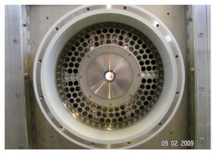
Figure 3: Post acceleration electrode assembly.
