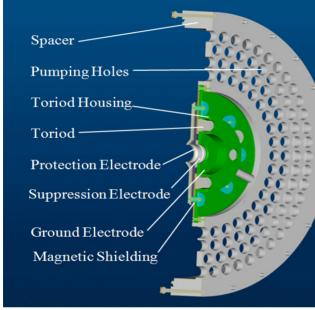
Figure 4: Sectional view of assembly.
