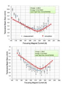
Figure 2: Envelope scan: Beam size measurements (crosses) versus solenoid current; triangle PARMELA simulation. Beam parameters : 1.28nC charge, ~5.5 MeV energy.
