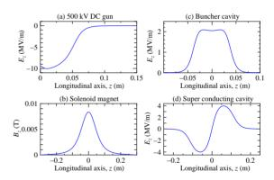
Figure 2: Field maps for the simulations of the cERL injector.
