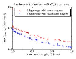
Figure 3: Optimization results with sector type magnets and rectangular type magnets. The emittance and the bunch length were calculated at 1 m from the exit of merger.
