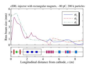
Figure 6: Horizontal, vertical and longitudinal rms beam sizes for the injector with rectangular type magnets.
