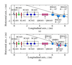
Figure 1: Layout of the cERL injectors with (a) sector bending magnets, and (b) rectangular bending magnets. Both the injection angles to the main linac are  $16^{\circ}$ .
