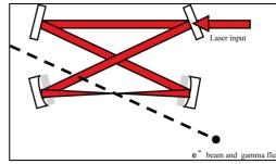
Figure 1: Geometry of the Compton collision for a four mirror optical resonator. The gamma flux will acquire the direction of the colliding electron beam.
