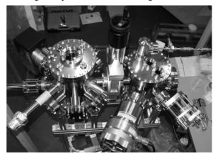
Figure 4: The loading (right) and the preparation (left) chambers of the 500-kV gun under an off-line test.
