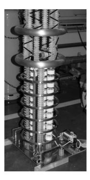
Figure 1: Cockcroft-Walton voltage multiplier for the 500-kV gun. The height is 1250 mm including the output registers on the top.
