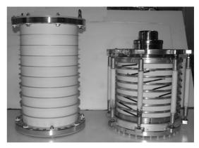
Figure 2: Multi-segmented ceramic insulator tubes for the old 250-kV JAERI FEL gun (right) and the 500-kV ERL gun (left). The guard rings are not installed at the 500-kV insulator.
