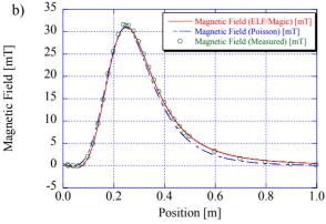
Figure 3: The solenoid magnet: a) cross sectional view; b) field distribution with backing coil adjusted to cancel the magnetic field on the cathode.
