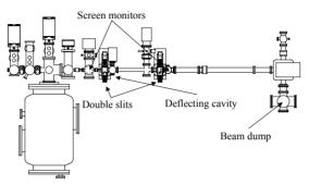
Figure 4: Layout of the beam measurement apparatuses.
