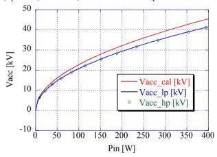
Figure 5: The deflecting voltage vs. RF input power. Blue dotted line, red line and solid circle are calculated value, low-power measured value and high-power measured value, respectively.
