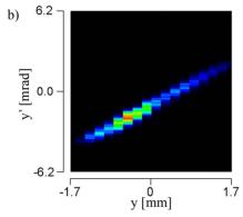
Figure 6: A typical result of initial emittance measurement: a) image on the screen of the beam that passed through the slit; b) reconstructed phase space plot.
