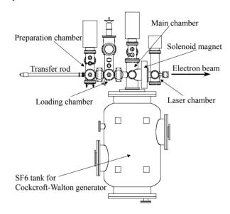
Figure 1: Top-view of the 250-kV, 50-mA photo-cathode electron gun.
