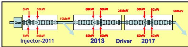
Figure 3: Schematic of e-Linac.
