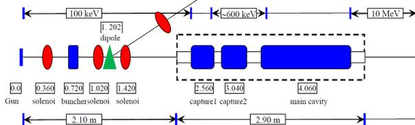
Figure 4: The 10MeV front end of the e-Linac.
