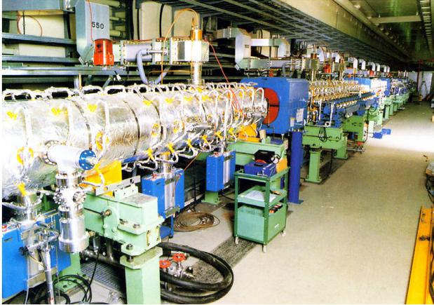
Figure 2: APS cavities installed in the TRISTAN main ring
