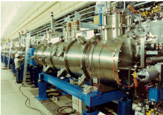
Figure 3: Superconducting RF system installed in the TRISTAN main ring.
