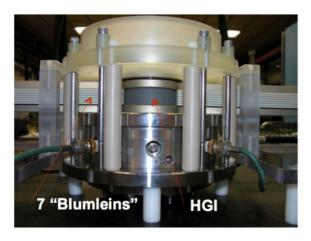
Figure 5: F.A.S.T. set up to accelerate electrons from a flashboard cathode. A 2.5 cm high HGI with a 4 cm bore is the wall of a diode. Two stacks of 7 "Blumleins" are shown feeding the HGI on either side. In some experiments, the diode was operated with a single stack. A sensitive beam current monitor is mounted below the HGI.
