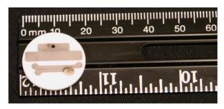
Figure 7: A spark discharge source provides the protons through a small aperture. Titanium electrodes are exposed to a hydrogen atmosphere to absorb the gas (two different sources are shown mounted on an alumina substrate). In operation, a pulsed high voltage is applied to cause a spark between adjacent electrodes that liberates hydrogen gas and forms a plasma. A series of powered grids is used to extract ions, suppress electrons and to gate the output pulse.
