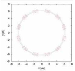
Figure 2: A tune-stabilized non-linear non-scaling FFAG lattice for protons 31 MeV to 250 MeV.
