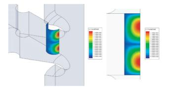
Figure 8: 14 MV/m electric field on inner rod for 5.9 MW, or 100 MV/m gradient.
