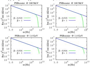
Figure 2: Comparison between the real (left) and imaginary (right) part of the transverse resistive wall impedance, for ultra relativistic approach [4] (-) and non ultrarelativiscit one (-) casting Eq. (4) in Eq. (5).
