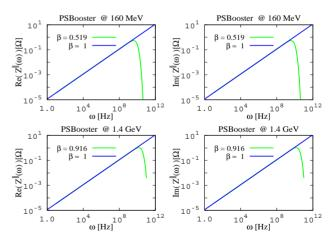
Figure 1: Comparison between the real (left) and the imaginary (right) part of the longitudinal resistive wall impedance, for ultra relativistic approach [4] (-) and non ultra relativistic one (-) Eq. (7).
