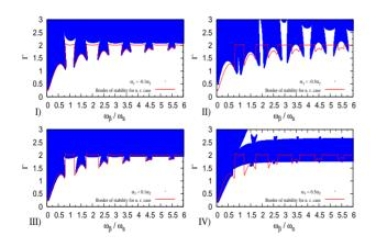
Figure 6: Stability region in the  $(\omega_\beta/\omega_s, \Gamma)$  plane for the two particle beam against the TMCI. The blue dotted regions (•) are those where the system is unstable. The red line (-) stands for the border of stability of the system at the ultra relativistic regime. The values used for the simulations are:  $\alpha_1 = -0.1\alpha_2$  plot I),  $\alpha_1 = -0.5\alpha_2$  plot II),  $\alpha_1 = 0.1\alpha_2$  plot III) and  $\alpha_1 = 0.1\alpha_2$  plot IV)
