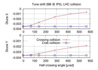
Figure 4: Horizontal detune (top) and vertical detune (bottom): crossing collision with one horizontal beam-beam element at IP5(H) (red); crab collision with the same beam-beam element at IP5(H) and two beams crabbed (blue).
