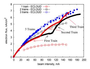
Figure 5: Electron flux comparison between the ECLOUD simulations (hollow squares) and measured at the e-detector (bold dots) for 1, 2 and 3 trains. The flux using ECLOUD simulations has been divided by 5 to show the results in the same plot.
