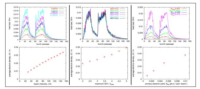
Figure 3: Top row: heat load evolution during one turn scanning the beam intensity (left),  $\delta_{\max}$  (middle), and  $N_{pe}$  (right). Bottom row: average electron density scanning the beam intensity (left),  $\delta_{\max}$  (middle), and  $N_{pe}$  (right).
