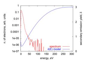
Figure 4: Energy spectrum obtained with the ECLOUD code for the case with  $\delta_{\max} = 3$ , and model of  $\delta(E)$ . The spectrum is dominated by electrons whose  $\delta(E) < 1$ .
